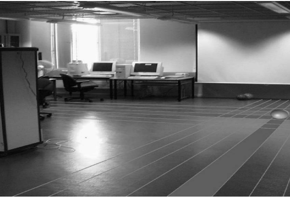
Fig. 2. The setting for EMFi sensor stripes under the laboratory's normal flooring. Some stripes are artificially visualized in the picture.
