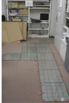
**Fig. 1.** Arrangement of binary sensor tiles.
