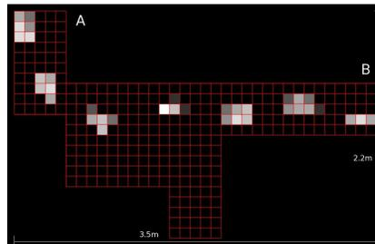
**Fig. 2.** Grey-level image calculated from sensor measurements of a walking sequence. In addition, the size of the sensor area is illustrated.
